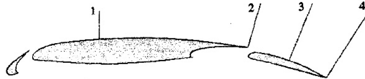
Figure 6.4: Geometry of the NHLP 2D airfoil with lines indicating the stations where total-pressure distributions have been measured. [From Hellsten (2005) — Copyright © AIAA 2005 — Used with permission.]
